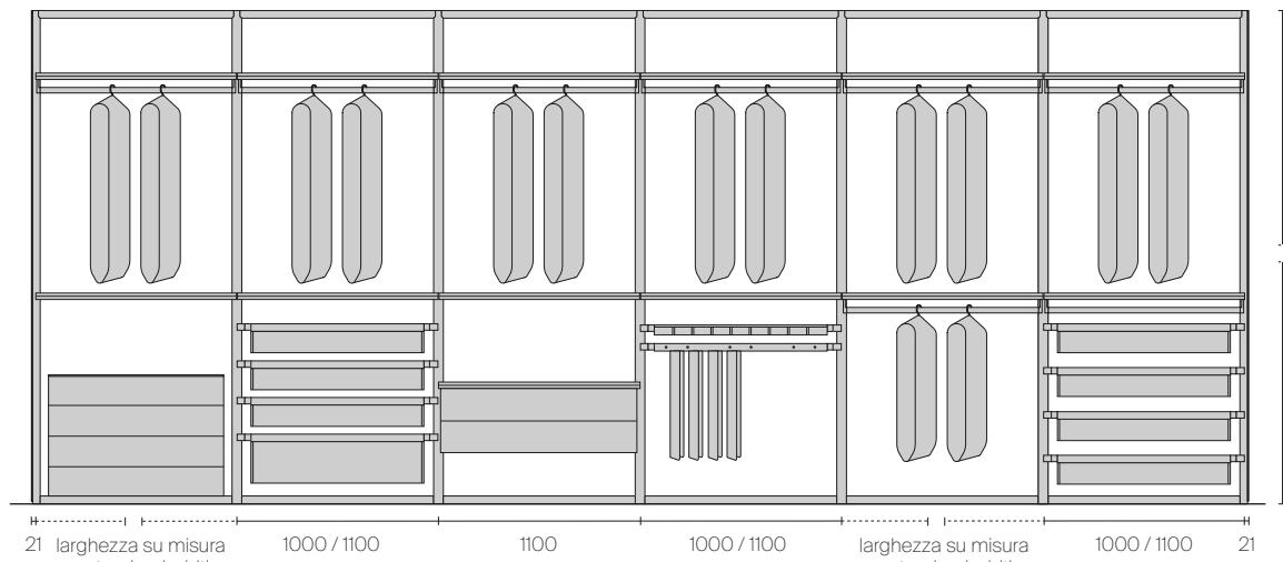
Fianco finale sp 48 mm, fianco intermedio sp 53 mm. Illuminazione a led opzionale anteriore e posteriore. Disponibile con rivestimento in vetro singolo frontale temperato sp 4 mm, Litech, tessuto, similpelle e essenza sahara / Closing side panel thickness 48 mm; middle frame thickness 53 mm. Optional front and rear led lighting system available with single 4 mm thick tempered glass, Litech, fabric, synthetic leather and sahara wood fronts
